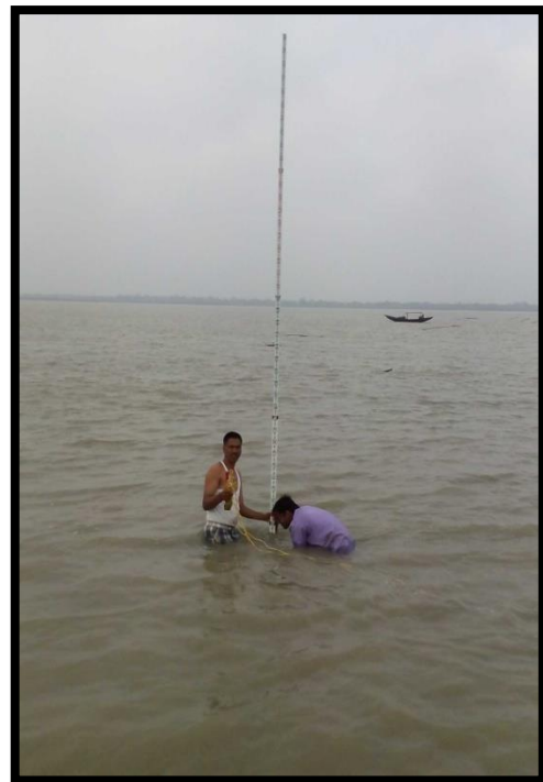
Tide Pole Erection At Chainage 0.28
