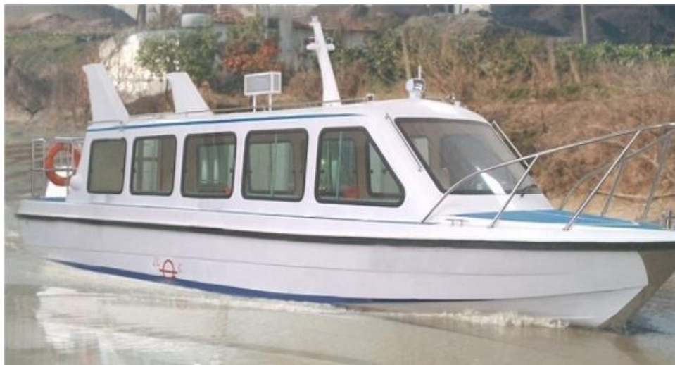
Figure 7-3: : Grandsea Fibreglass 30 Pax Water taxi / Passenger Boat
