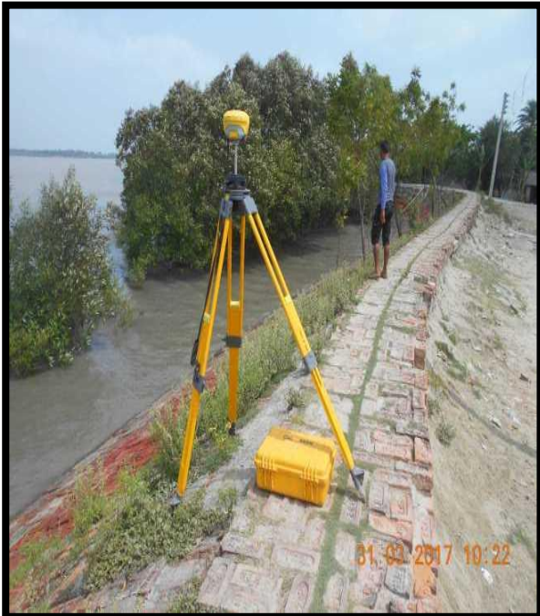
BASE STATION AT CHAINAGE 74.5, RIGHT BANK
