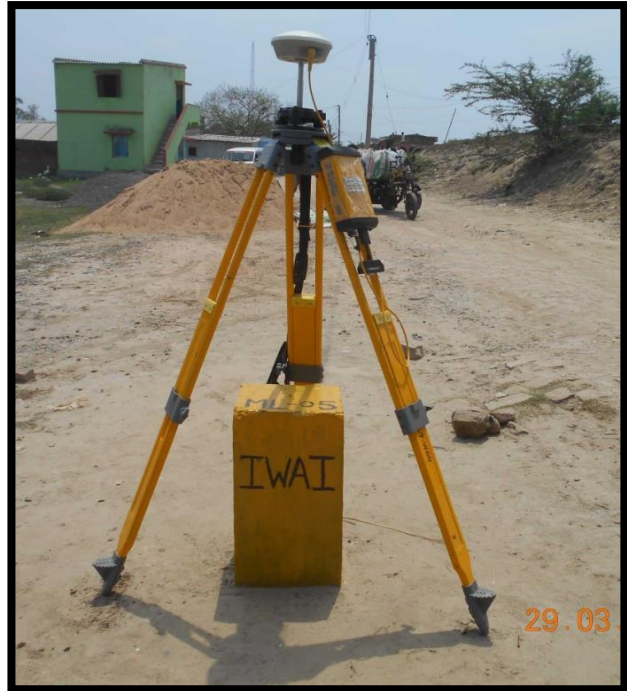
BASE OBSERVATION ON ML-05 AT CHAINAGE
