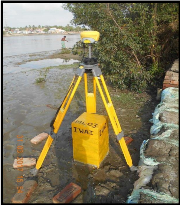
BASE STATION ML-03 AT CHAINAGE 80.5, RIGHT BANK
