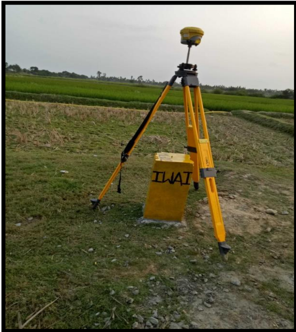
BASE OBSERVATION AT ML-02 AT CHAINAGE 69.7
