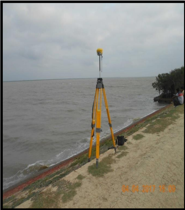
BASE STATION AT CHAINAGE 57.5 , LEFT BANK
