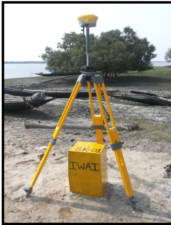
DGPS Observation at BM SK-01at Chainage 5.1
