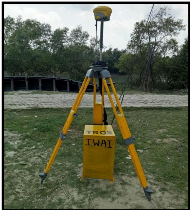
GPS Observation at Left Bank TR-05 At Chainage 40
