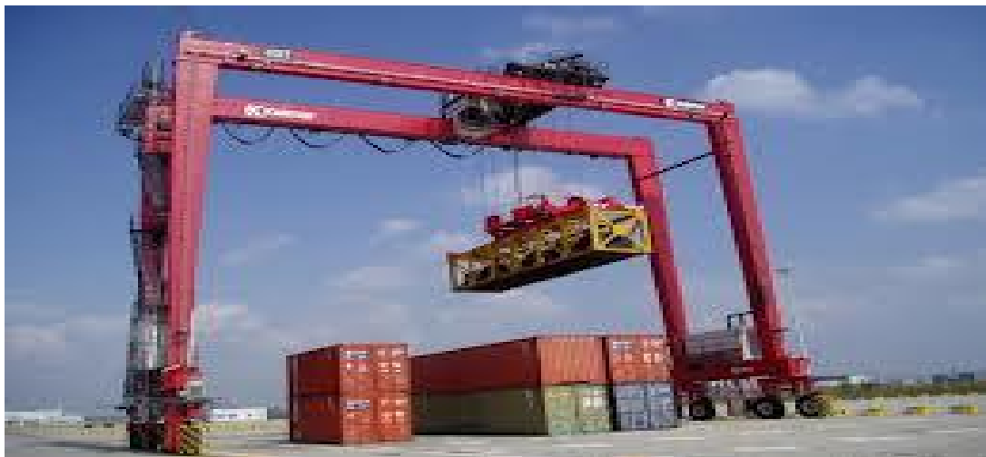
Fig 11– 7 Rubber Tyre Gantry Crane
