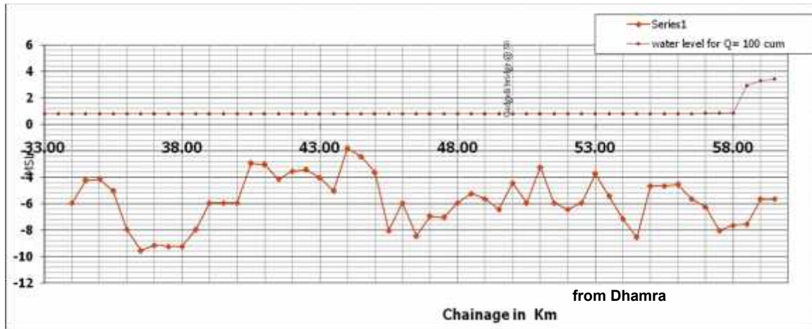
Figure No. 6-3 Water Surface Profile along Kharsua 60 to 105 Km (Padanipal to Mangaladi) – Model run for Q = 100 cum/sec
