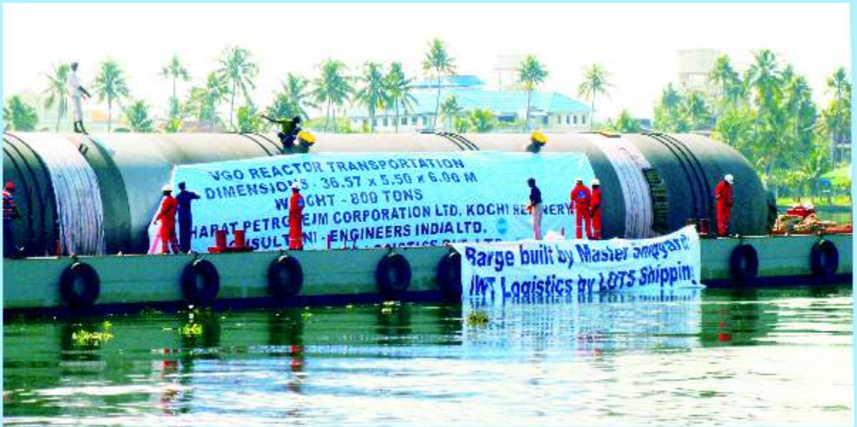
movement of 800 MT VGO reactor to Koch refinery in NW3
