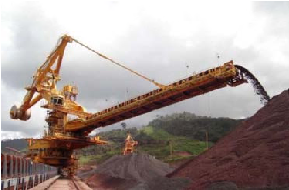
Figure : Typical Arrangement of Stacker
