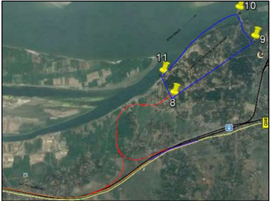
Figure 8.4: Y shape Connection with IWT terminal at Sahibganj
