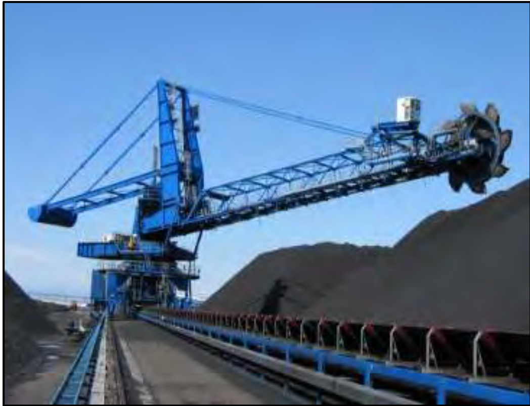
Figure 10.7: Typical Bucket Wheel Reclaimer
