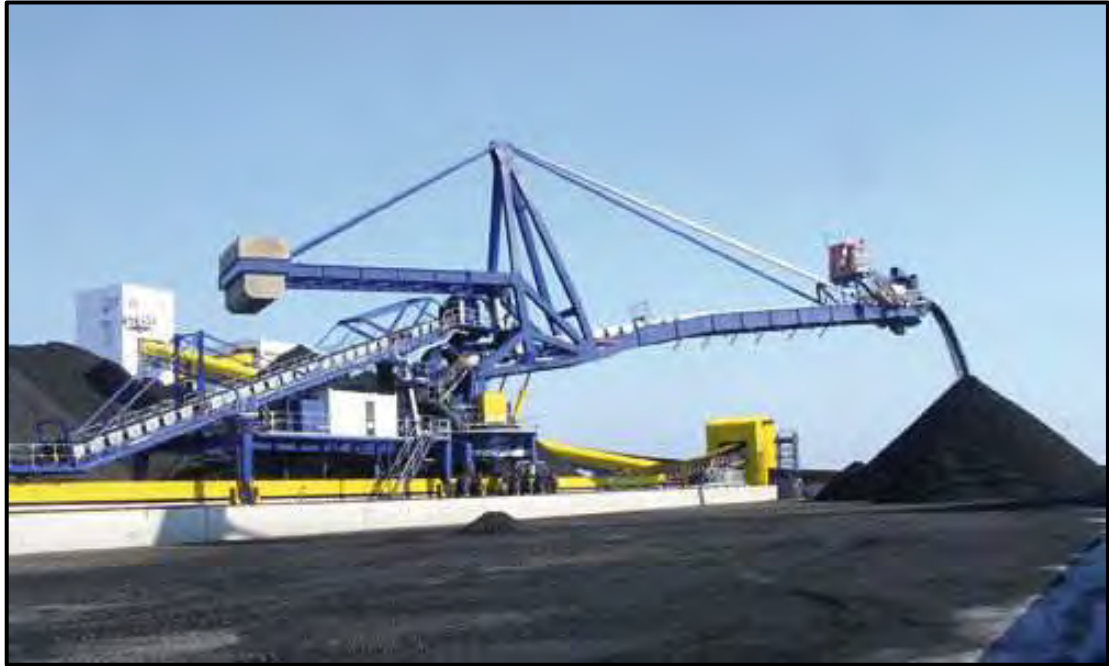
Figure 10.6: Typical Arrangement of Stacker cum Reclaimer
