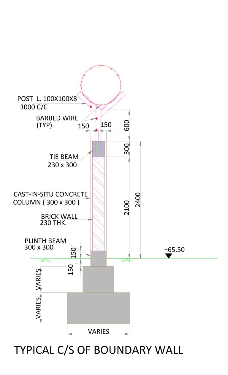
**BOUNDARY WALL** PROPOSED TERMINAL AREA **KEY PLAN** LEGEND: PROPOSED TERMINAL AREA NOTES: 1. ALL DIMENSIONS ARE IN MILIMETRE 2. ALL LEVELS ARE IN METRE & ARE WITH RESPECT TO MSL INLAND WATERWAYS AUTHORITY OF INDIA TENDER FOR ENGINEERING, PROCUREMENT AND CONSTRUCTION OF INTER-MODAL TERMINAL FOR IWT AT GHAZIPUR 26-09-17 26-09-17 HOWE 26-09-17 IWT TERMINAL AT GHAZIPUR -TYPICAL JOB. NO. DRG. NO. I-525 GPT-1019 DETAIL OF BOUNDARY WALL WITH FENCING
