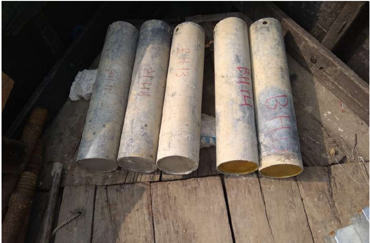
Figure 3: Wax sealed undisturbed samples
