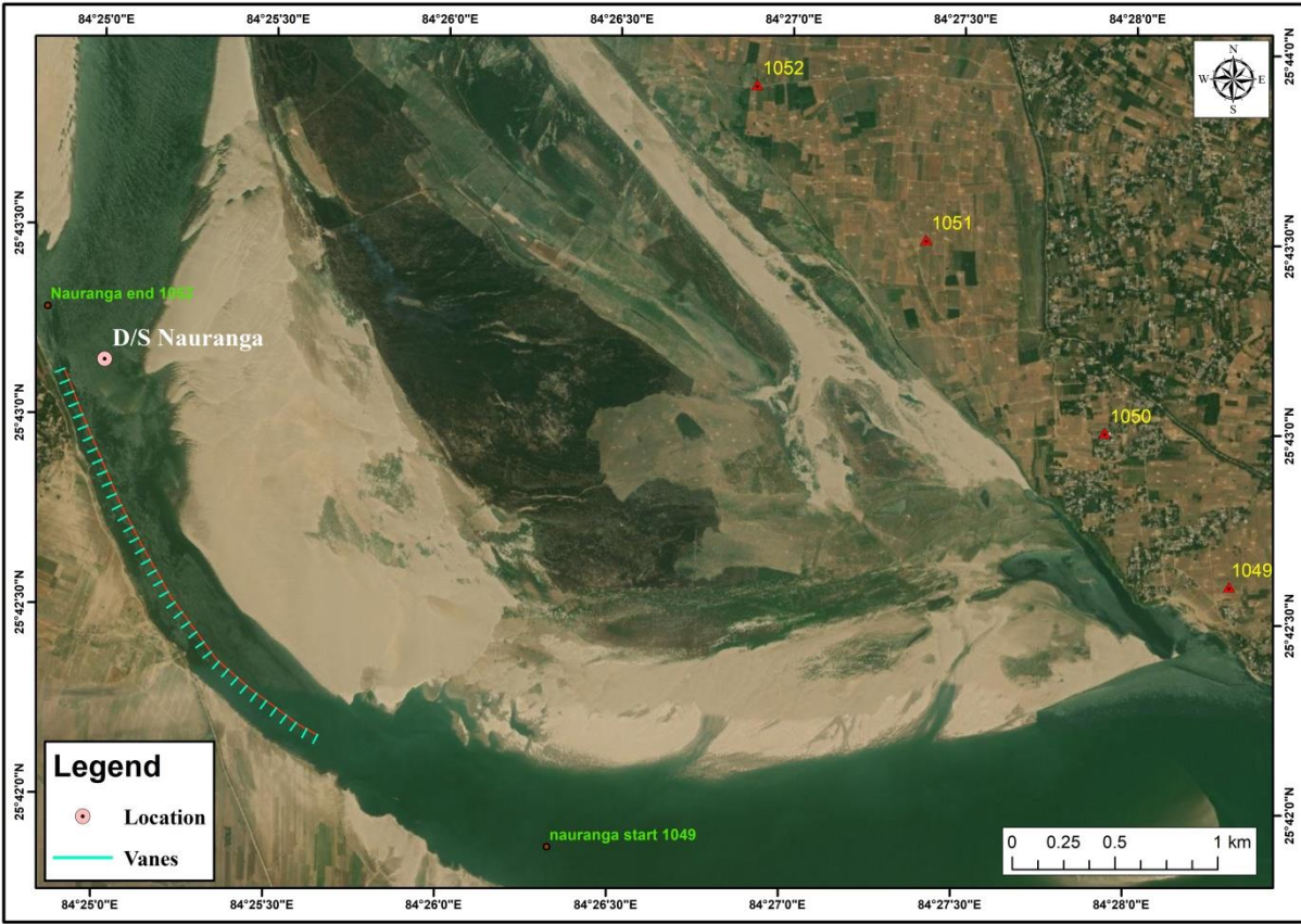
Proposed submerged vanes at Nauranga reach
