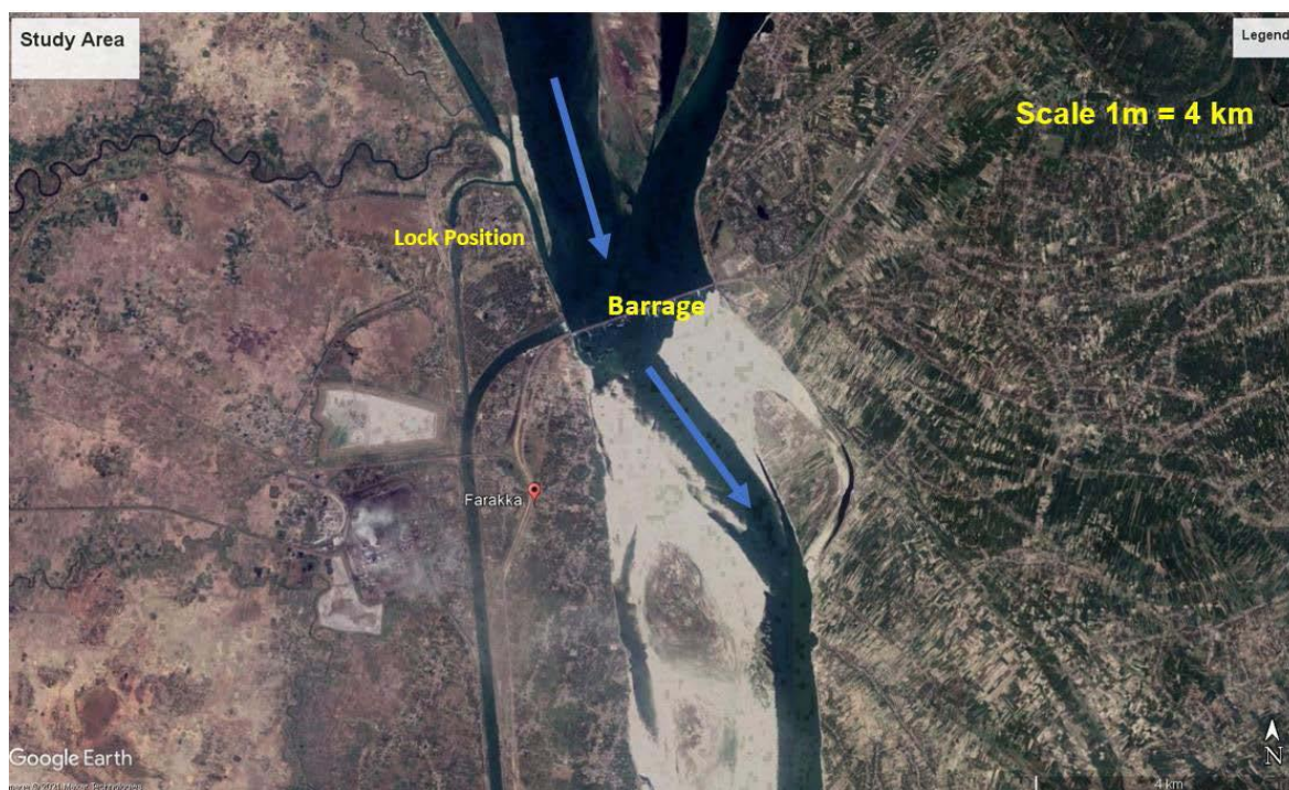
Figure 2 Plan Map of Farakka Barrage and Navigational lock
