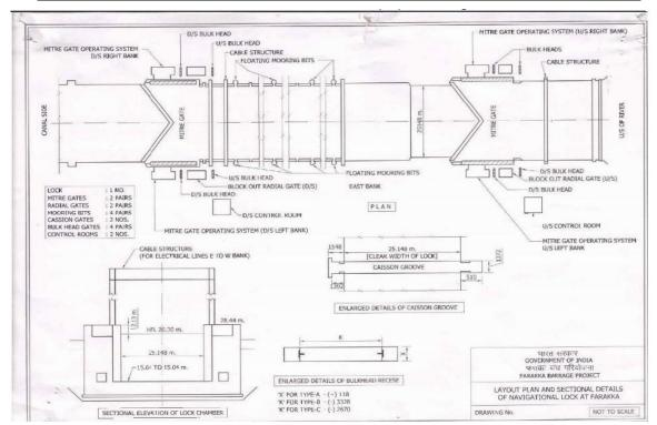
Figure 1.4 Layout of the existing Navigational lock
