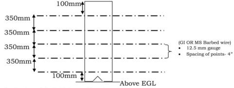
5 nos. barbed wire with 0.350mtr. Spacing Total = (10mtrX5nos.) = 50 rmt.
