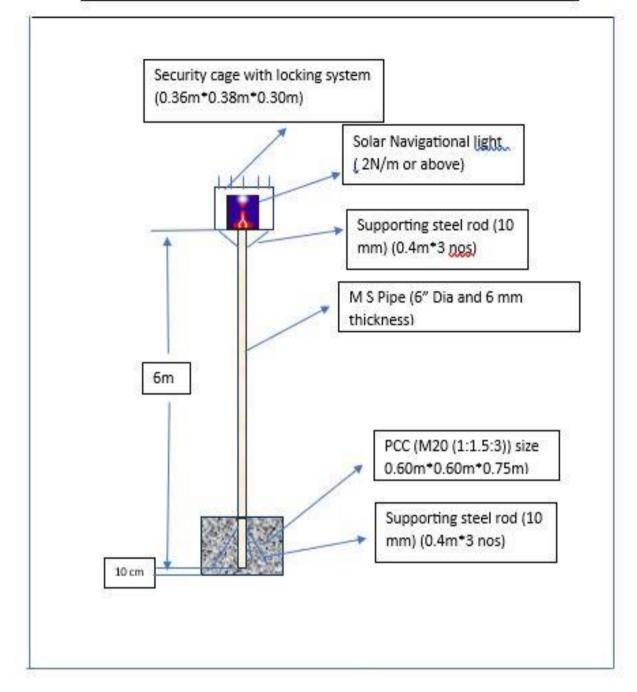
DRAWING OF 6 M HEIGHT BEACON TOWER WITH M.S. PIPE
