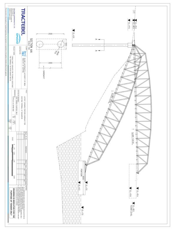
This is a conceptual drawing (size 30 m x 2 m x 2.2 m) and as per Design the gangway to be fixed with a vertical variation of 10.5m during flood and lean season.
