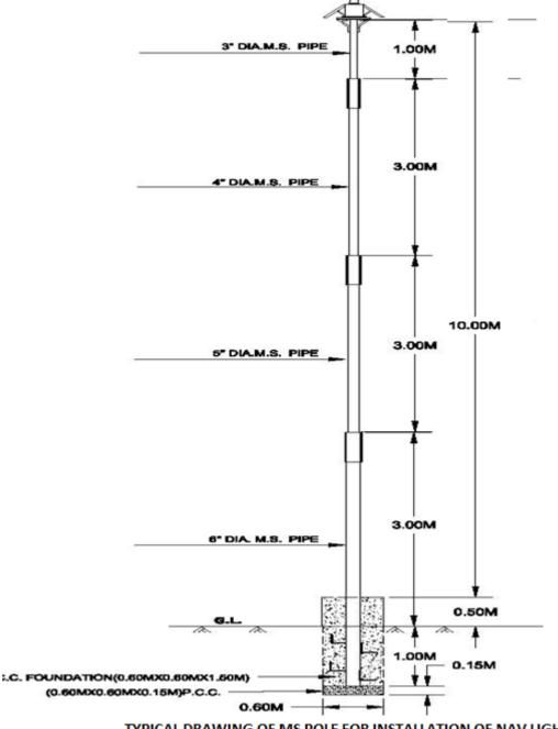
TYPICAL DRAWING OF MS POLE FOR INSTALLATION OF NAV LIGHT
