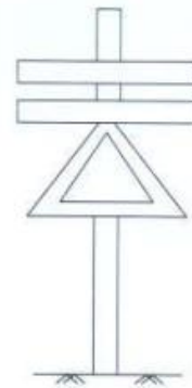
PARI HATH (LEFT HAND MARK TRANSIT) COME TOWARDS ME AND LEAVE ME ON RIGHT WHILE GOING ON UPSTREAM
