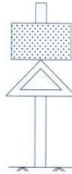
PARI MUNDA (RIGHT HAND MARK TRANSIT) COME TOWARDS ME AND LEAVE ME ON LEFT WHILE GOING ON UPSTREAM
